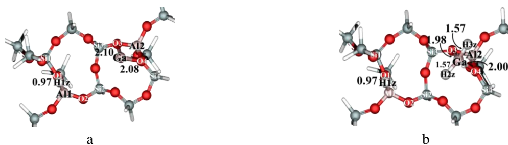
Figure 1. Optimized structures of 14T models of a) Ga/H-ZSM-5 and b) GaH 2 /H-ZSM-5.
